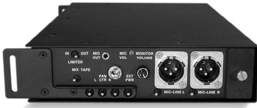
1. Mic Volume – The trim pot marked MIC VOL is a screwdriver slate mic gain control adjustment.
