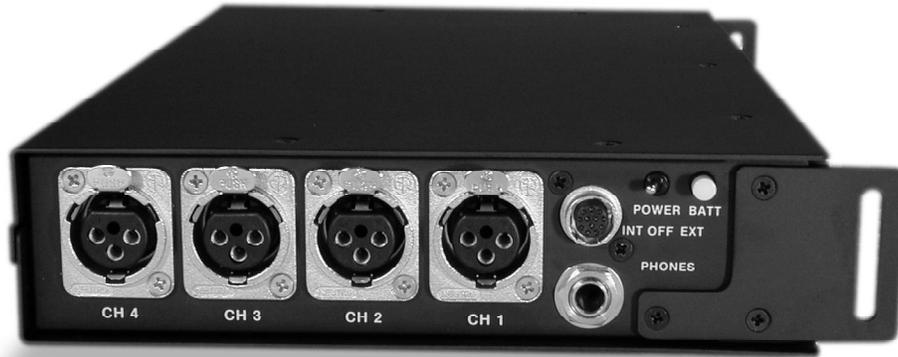
1. Mic Inputs, Channel 1 – 4 – The XLR mic inputs are electronically balanced where pin 1 is shielded ground, pin 2 is input high, and pin 3 is input low. Either pin 2 or 3 may be tied to ground.
