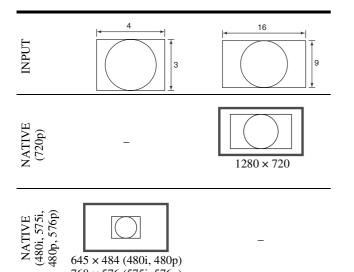
To display in 4:3 aspect ratio, images are adjusted horizontally with scale handling.
