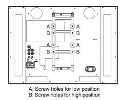
**3** Attach the stand attachment bracket with four screws.
