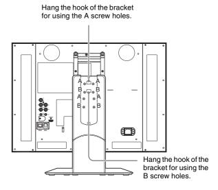
**5** Secure the arm with four screws.
