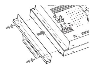
**2** Attach the unit to the rack with four screws.
