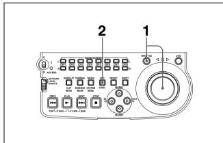
**1** Hold down the SHUTTLE button, and turn the jog dial or shuttle dial.
