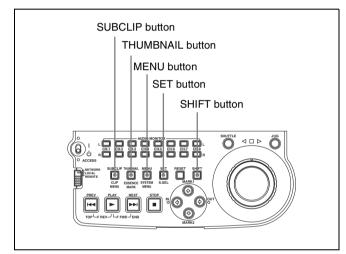
With the THUMBNAIL button off, hold down the SHIFT button and press the SUBCLIP button.
