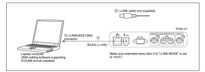
For the method of transferring video/audio signals (AV/C data) to a nonlinear editing system, refer to the manual provided with the editing software to be used.
