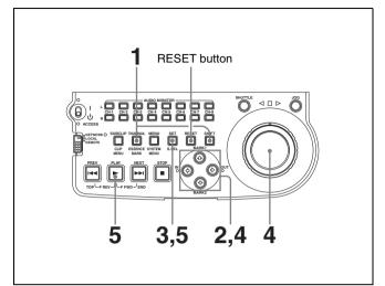
**1** Hold down the SHIFT button, and press the THUMBNAIL button, turning it on.
