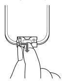
2 Set lithium battery in the case so that the + symbol on the battery is facing you.
