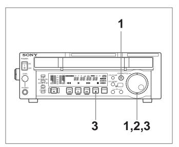
In shuttle mode, the SHUTTLE dial controls the playback speed based on the angular position of the dial.
