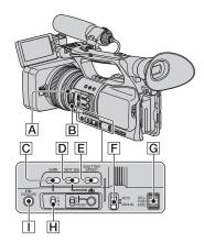
You can adjust the image brightness by adjusting the iris, gain or shutter speed, or by reducing the light volume with the ND filter B. Also, when [EXPOSURE] is assigned to the iris ring A, you can adjust the iris, gain and shutter speed with the iris ring A. You can assign [IRIS] or [EXPOSURE] to the iris ring A from [IRIS/EXPOSURE] of the [CAMERA SET) menu (p. 69). The default setting is [IRIS].
