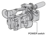
1 Slide the POWER switch to CAMERA or VCR while you press the green button.
