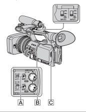
1 Set the AUTO/MAN (CH1/CH2) switch A of the channel to be adjusted to MAN.
