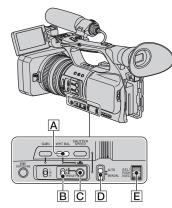
You can adjust and fix the white balance according to the lighting conditions of recording environment.
