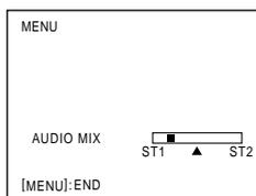
Five minutes after when you disconnect the power source, the setting of AUDIO MIX returns to the original sound (stereo 1) only. The factory setting is original sound only.
