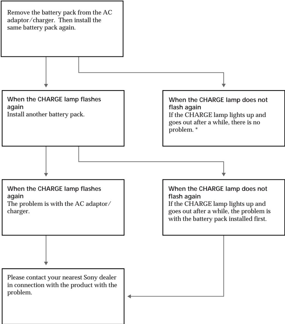
\* If you use a battery pack which you have just bought or which has been left unused for a long time, the CHARGE lamp may flash at the first charging. This does not indicate a problem. Repeat again to charge with same battery pack.
