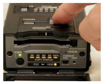
Formatting HDD is started by hitting START key during orange LEDs , COPY STATUS, are blinking. Formatting is finished when LEDs are turned off.
