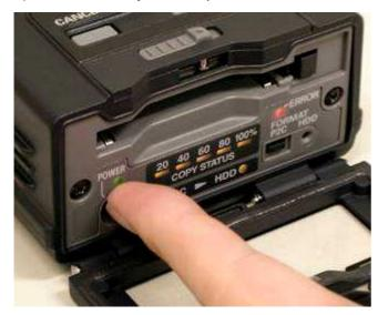
All LED flash two times, then power LED brink 10 seconds during boot up hard disk. After hard disk is ready, Power LED turns to ON.
