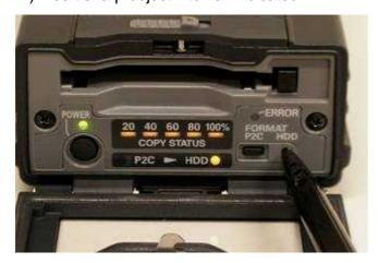
Formatting disk is required in order to erase data in HDD.
