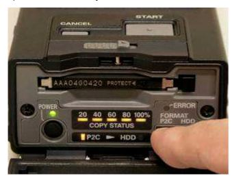
Format P2card for erase all material. COPY STATUS LED is blinking at orange by pressing "P2C" key more than two seconds.
