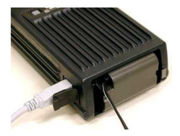
AC adaptor is recommended when operating with PC in order to avoid accidental shut down.
