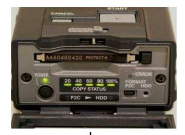
Copy process is finished when copy status LEDs are all ON.
