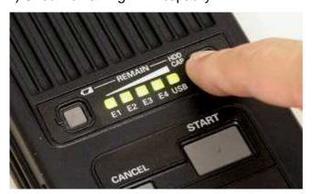
Five LEDs indicate remaining disk capacity when press "HDD CAP." key.
