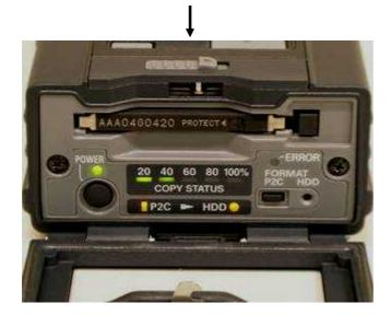
Orange lights is ON at "P2C > HDD" and copy progress is indicated by five green LED from 20% to 100%.
