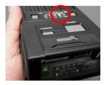
During protect disk, LED "E4" is turned to Orange. When shock or vibration is stopped, orange light is turned off, and start writing again in a few seconds.
