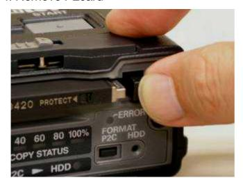
Press Eject button once. The knob is come out, then press Eject button again, P2card is ejected.
