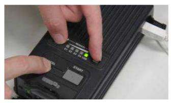
Press continuously both side of keys in STATUS area and Cancel key simultaneously until USB LED is turned to Orange. Set up is done when USB LED is turned to orange.
