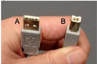
Use typical USB cable which has A and B connectors such as left picture.
