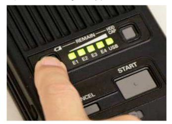
By pressing left side key, LEDs indicate remaining power of battery. We recommend full charges before use.
