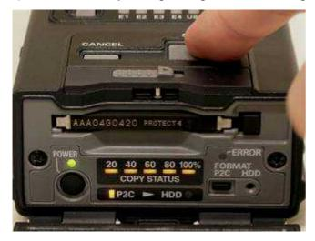
P2card formatting is started when hit START key during orange LEDs are blinking. Format is finished when LEDs turn off.
