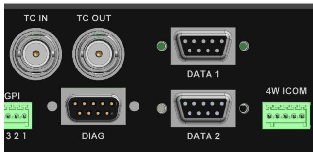
Figure 14 - Two Bi-Directional Data Channels
