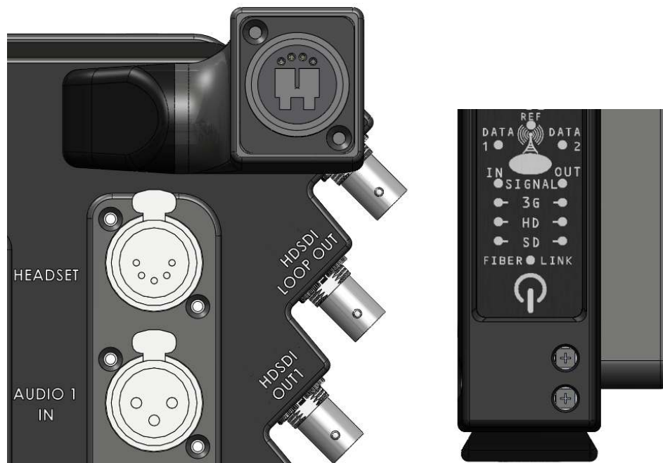
Figure 3 - Camera Video Connectors and Status
