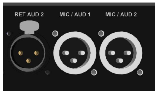
Figure 12 - MIC/Line Audio 1 and 2 Outputs
